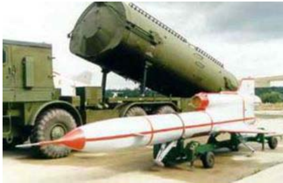
Tu-143 on transporter-erector-launcher (TEL)
