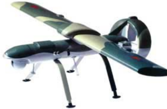
Pchela-1K modernized version of Shmel-1. Note the lack of turned down wingtips
